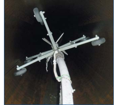
(RIGHT) The Tunnel Cleaner can be adjusted to fit a range of pipe sizes (1.2 - 3.6m dia).
