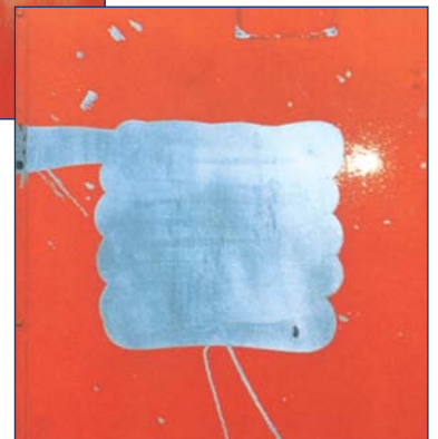
(RIGHT) Removing 1ft² of coating from an aluminum vessel in just 24 secs. That's 14m²/hr (150ft²/hr)!
